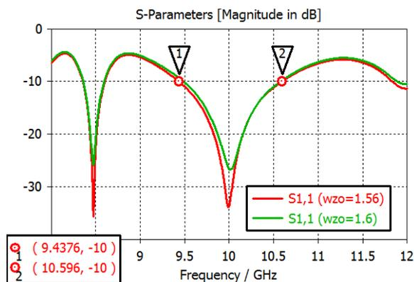
Fig. 9 Frequency characteristics of return loss.
