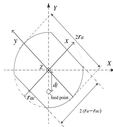
Fig. 3 Dimension of feeding element.
