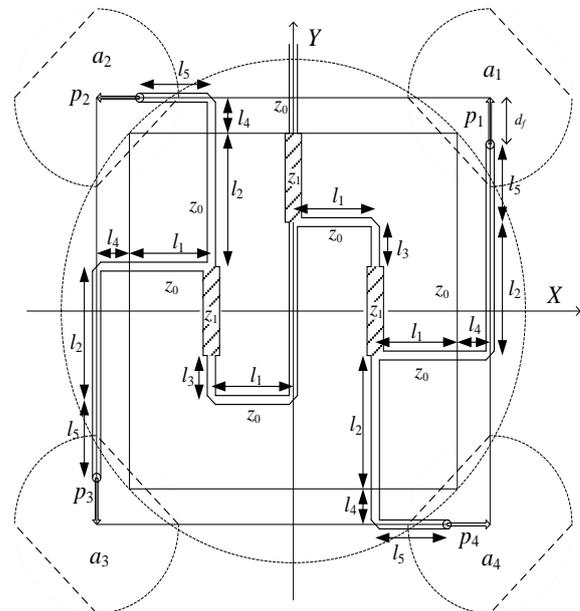
Fig. 8 Routing wire pattern for the proposed array antenna with 4 unit antennas.
