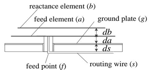
Fig. 2 Cross-sectional view of the proposed antenna.
