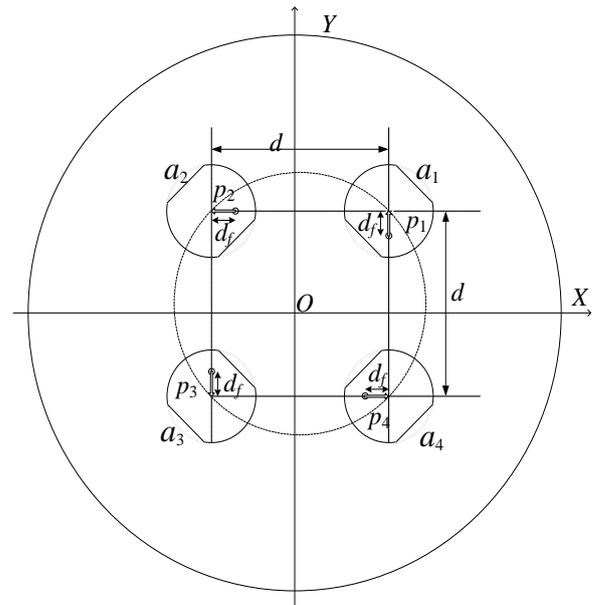
Fig. 7 Configuration of plane array antenna. Reactance elements and dielectric substrate are abbreviated.
