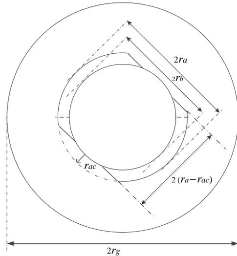
Fig. 1 Overhead view of the proposed antenna. The dimension of reactance element is included.
