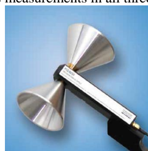
Fig.2 PCD- 8250 precision dipole antenna
