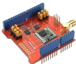
Figure 5: SX127x LoRa Shield
