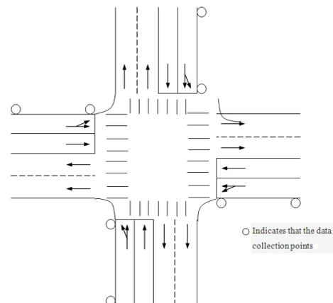
Fig.2 Schematic of traffic flow data collection
