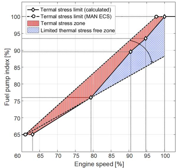
**Fig. 5.** Calculated and sloped linear characteristic for thermal stress limit
