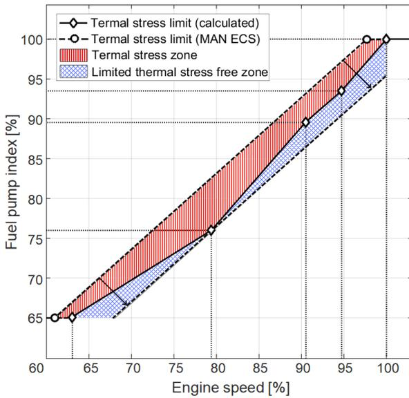
**Fig. 3.** Calculated and used linear limiting characteristic moved parallel downward
