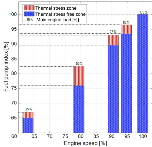
**Fig. 2.** Comparison of fuel pumps indices with the used and calculated limiting characteristics of a diesel engine in terms of thermal stress
