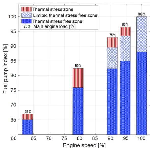
**Fig. 6.** Comparison of the fuel pumps indices with the calculated and used linear limiting characteristic with a modified slope
