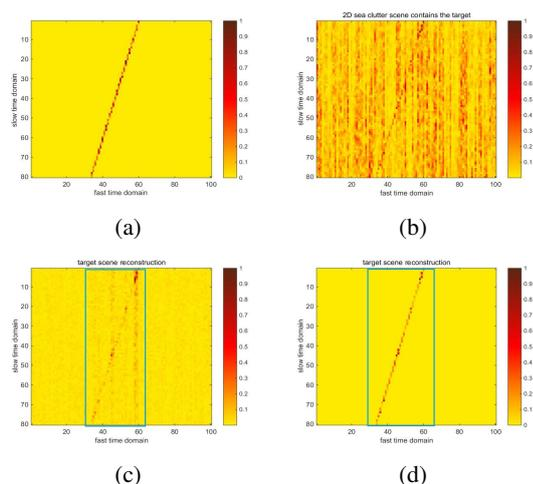
Figure 3: Example of target localization and reconstruction in sea clutter. (a) Simulation of the target trajectory. (b) Target amid the clutter. (c) Results using orthodox STAP algorithm. (d) Results using proposed method on the test set.
