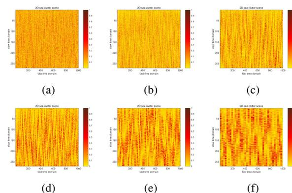
Figure 2: Example of sea clutter scene simulated by K-distribution. (a) sea state degree 1: Very Low (short and low wave) (b) sea state degree 2: Low (long and low wave) (c) sea state degree 3: Light (short and moderate wave) (d) sea state degree 4: Moderate (average and moderate wave) (e) sea state degree 5: Moderate rough (long and moderate wave) (f) sea state degree 6: Rough (short and heavy wave).
