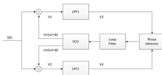
Fig. 1 Block diagram of Costas Loop
