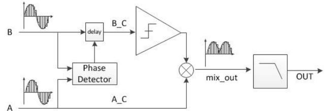
Fig. 2 Block diagram of proposed circuit
