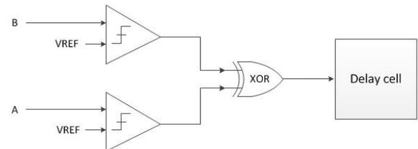
Fig. 3 Phase Detector circuit
