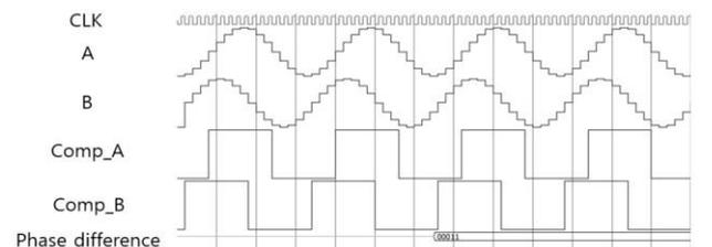
Fig. 4 Wave of Phase Detector circuit
