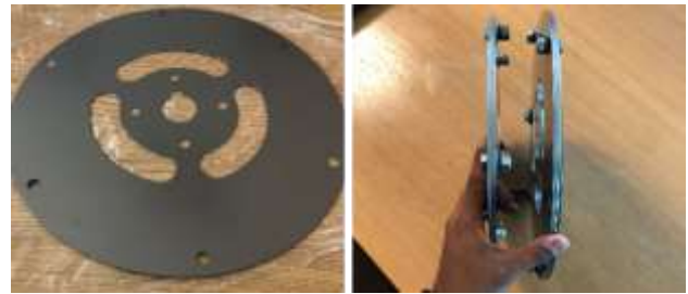
Fig. 6. Stacking of rotor laminations.
