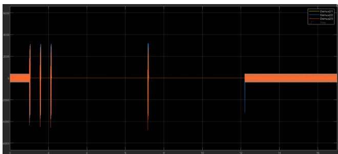
Fig. 31 Line current behavior for Scenario 2 where a temporary 2LG fault occurs and the relay system acts to clear the fault
