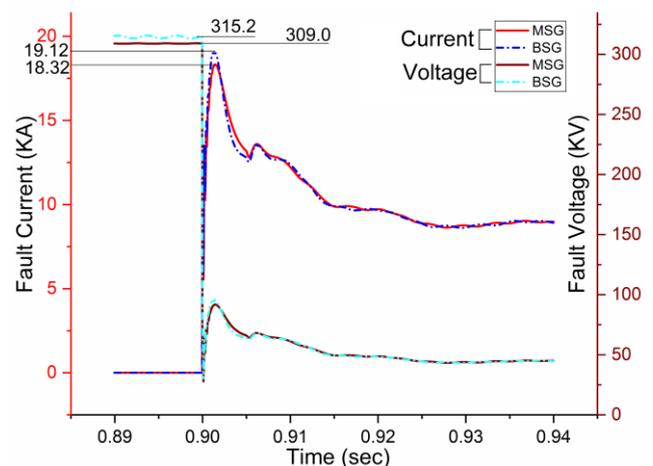
Fig. 11. Monopolar Vs Bipolar Pole to Ground fault
