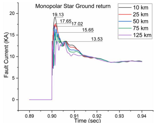
Fig. 14. Effect of distance over P-G fault in Monopolar Star Ground return
