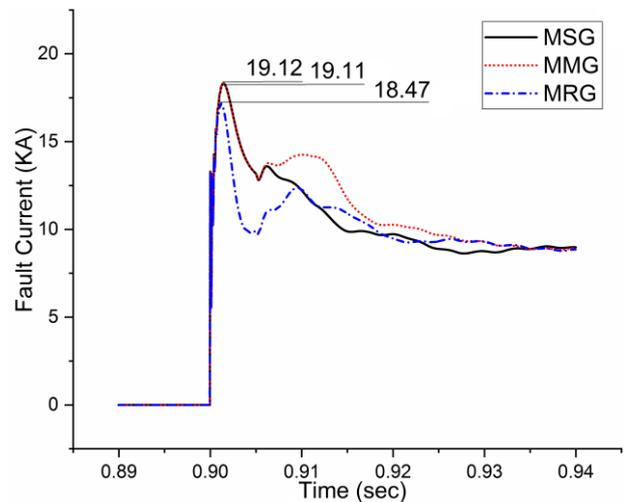
Fig. 13. Mesh, Star and Ring Sections fault response in Bipolar Ground return
