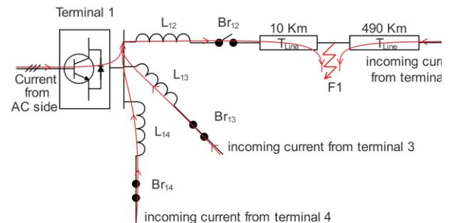
**Fig. 9. Fault current flow**
