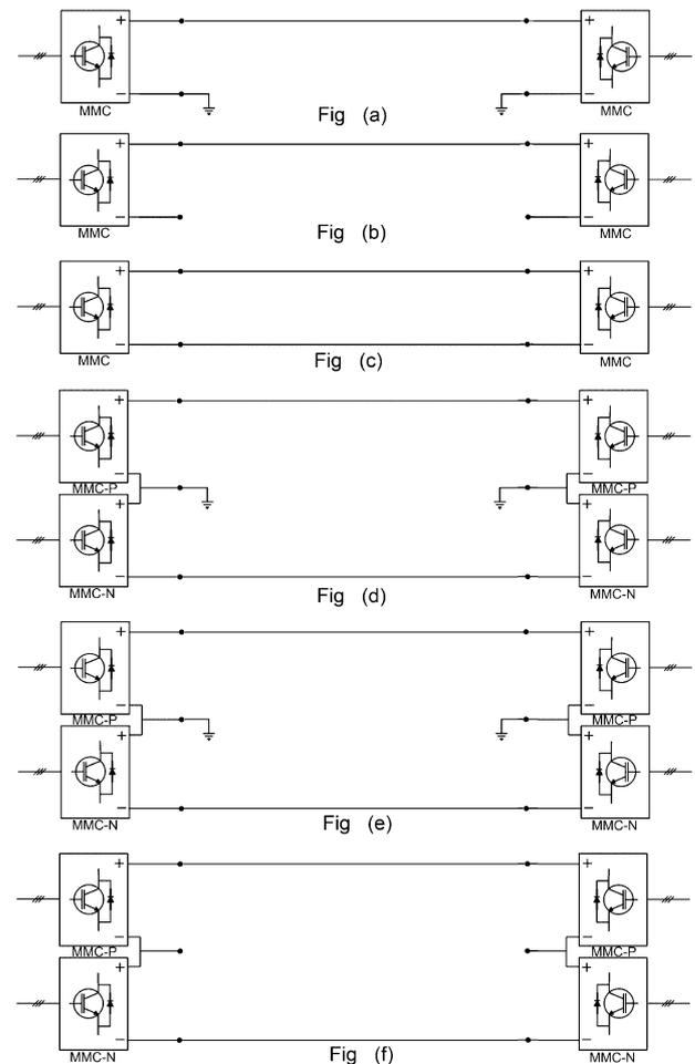
**Fig. 1. Polarity and Return Path**
