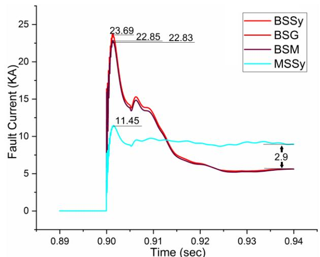
Fig. 15. Pole to pole fault response in monopolar star symmetric topology and bipolar star design for different returns
