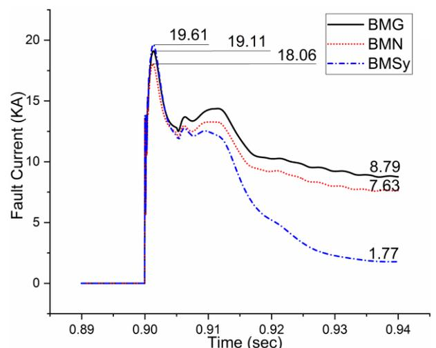
Fig. 12. Fault Current for Bipolar Mesh design Ground, Neutral and Symmetric return
