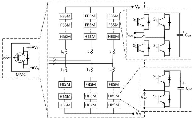
**Fig. 3 Hybrid VSMMC in test circuit**
