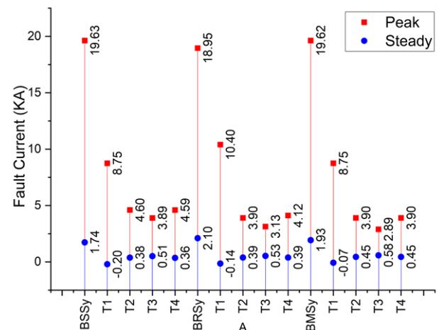
Fig. 17. Transient and Forced Response in Bipolar Symmetric return topologies with current observed at terminals
