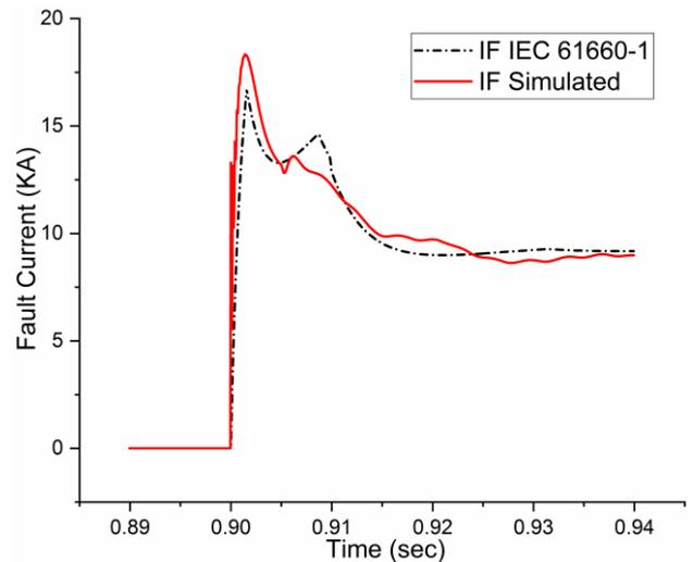
Fig. 10. Simulated vs IEC 61660-1 P-G fault (dash) in Monopolar Star Ground return topology
