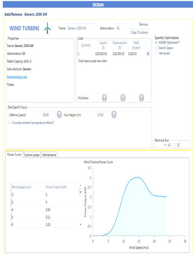
Figure 4: Wind Turbine Generator
