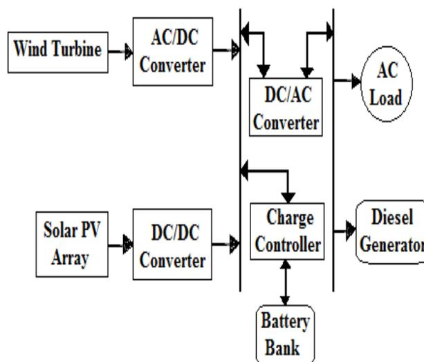
Figure 2: Design of Hybrid Distributed Generation System
