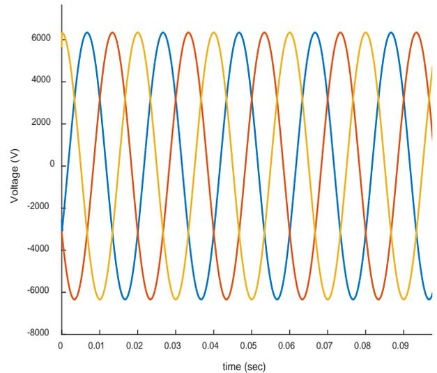
Fig.3: Voltage waveform during no fault condition.
