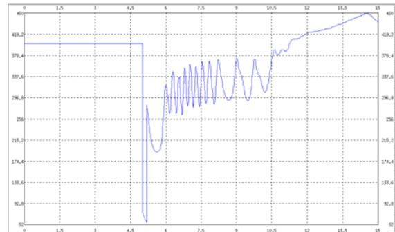
Fig. 9. Voltage at the level of SKS group 2 substation 400 kV.
