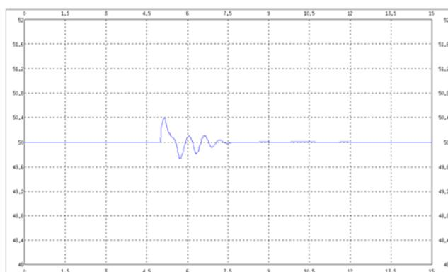
Fig. 18. Frequency at the level of SKH group 3 substation 400 kV.
