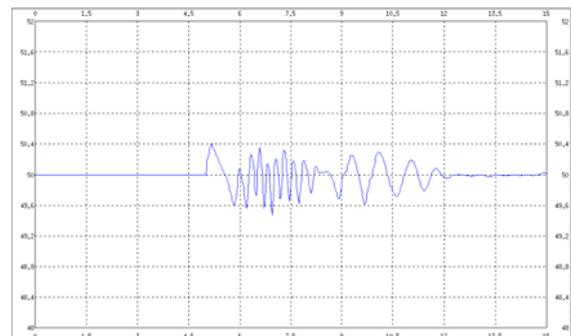
Fig. 10. Frequency at the level of SKS group 2 substation 400 kV.
