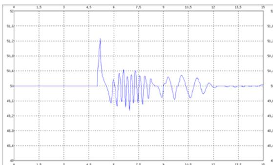
Fig. 8. Frequency at the level of SKS group 1 substation 400 kV.
