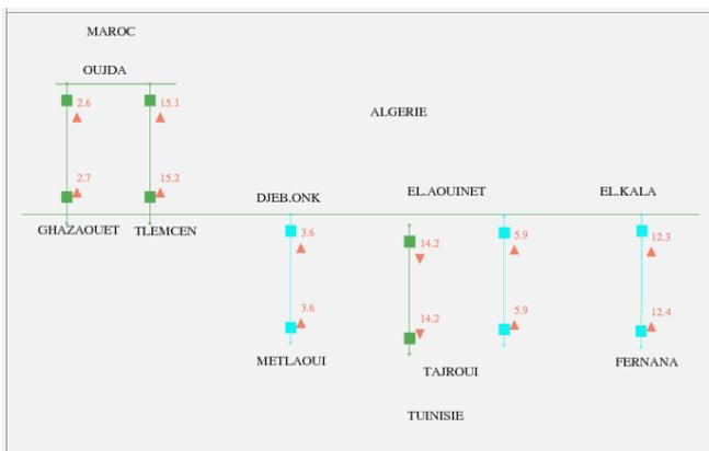
Fig. 3. Active transits on the interconnection lines Algeria –Morocco and Algeria-Tunisia (normal situation)
