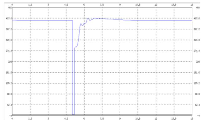
Fig. 17. Voltage at the level of SKH group 3 substation 400 kV.
