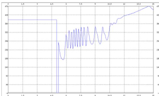
Fig. 7. Voltage at the level of SKS group 1 substation 400 kV.
