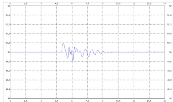
Fig. 16. Frequency at the level of SKH group 3 substation 400 kV.
