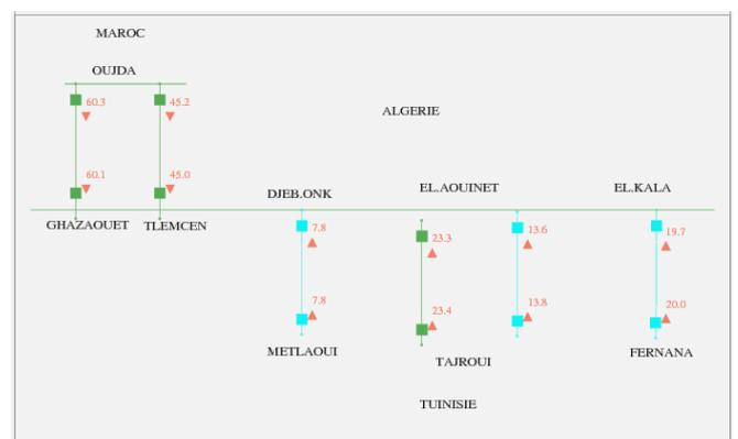
Fig. 4. Active transits on the interconnection lines Algeria-Tunisia and Algeria-Morocco ( Loss of a CC 400MW)
