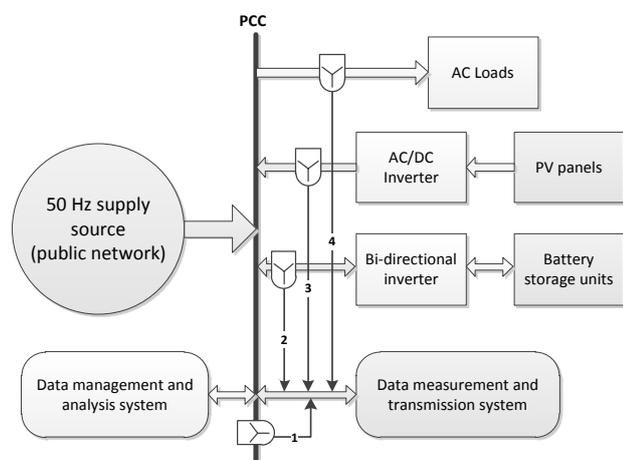
Fig. 2. Schematic of AC-connected hybrid energy system of SGRL
