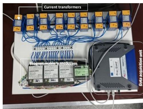
Fig. 3. Connection configuration of the remote data acquisition and transmission units
