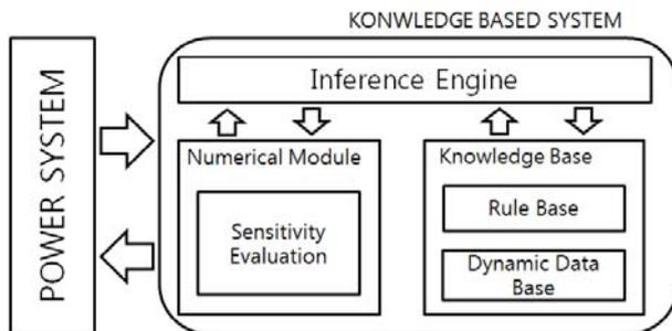
**Fig. 2.** Structure of intelligent voltage control system
