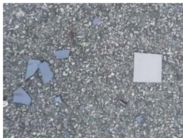
Fig. 5. Drop test results of two magnetic bodies
