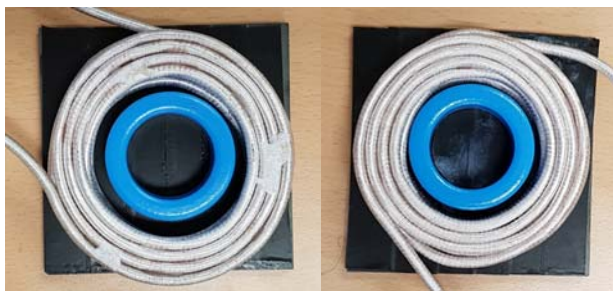
Fig. 2. Transmitting(left) and receiving(right) coils. The Litz wire used in coil fabrication is 0.12 mm thick and has 300 strands. Both coils have a diameter of 9.7 cm and have a turn number of 16 turns. The transmission side magnetic body used the conventional magnetic ferrite, while the receiving side magnetic body alternately tested the conventional ferrite and the proposed SMC.
