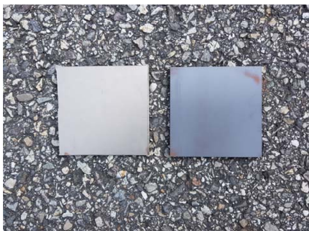
Fig. 3. The developed SMC (left) and conventional ferrite (right)
