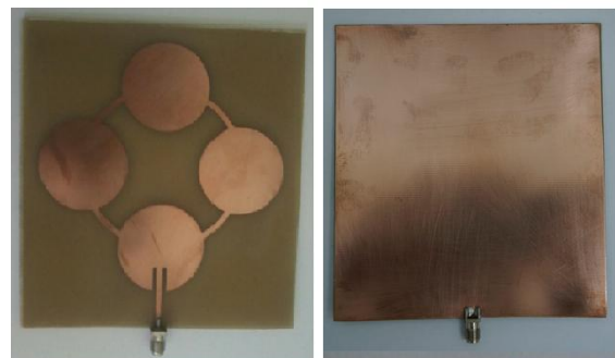
Fig. 8 Picture of the circular array
