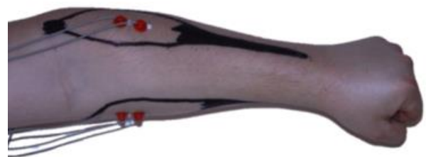
Fig.2: EMG electrodes placed on the arm (Source: authors)
