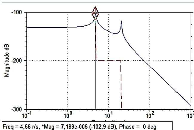
Figure 11. Bode Plot and Natural Frequencies of Vertical Motion
