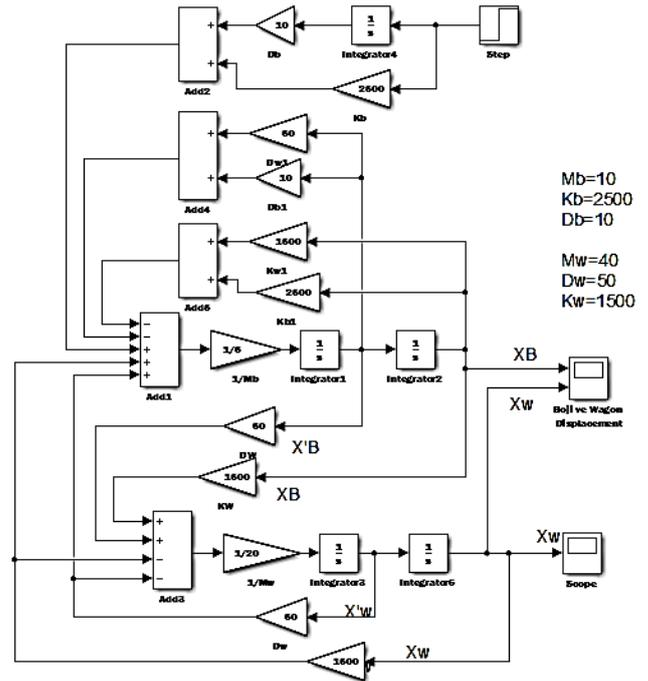
Figure 9. Simulink simulation of vertical suspension motion
