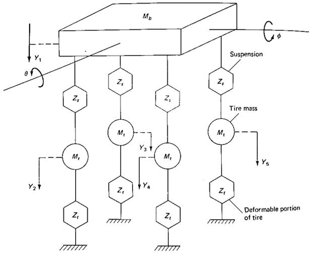
Figure 7. Seven degree of freedom track suspension network models
