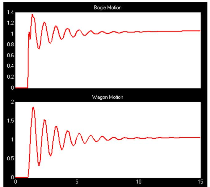
Figure 10. Time response of Bogie-Wagon
