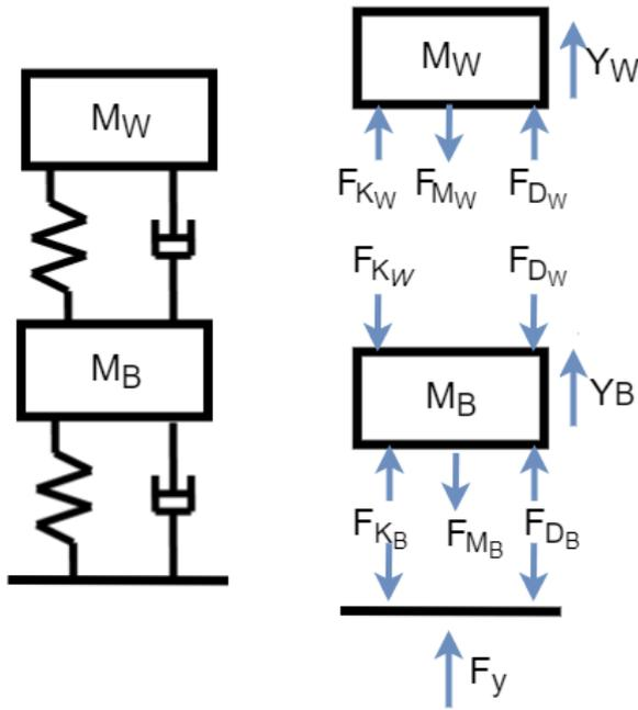
Figure 8. Bogie-car model with free-body diagram.
