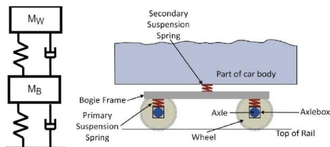
Figure 2. Mathematical model of bogie-chasse construction.
