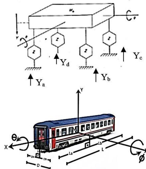
Figure 6. Three Degree of Freedom Network Suspension Model.
