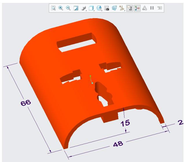
*Fig 2: Three-Dimensional Model of Electric Socket Adaptor*
