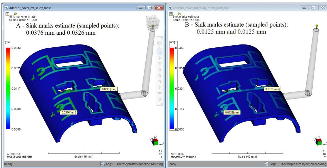
Fig. 7: Comparison of Sink Marks Estimate with default Packing Profile (left) and Optimised Packing Profile (right)
