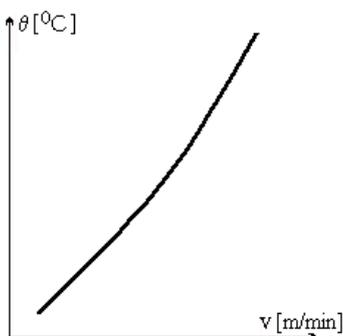
Figure 13 Temperature variation with cutting speed
