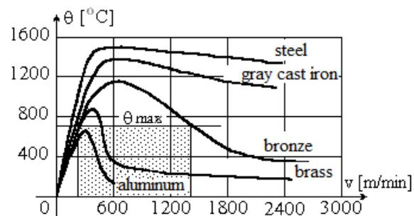
Figure 10 Influence of cutting speed on cutting temperature
