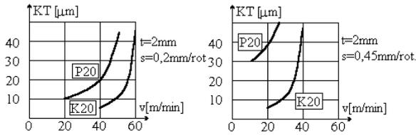
Figure 6 The wear on the front face
