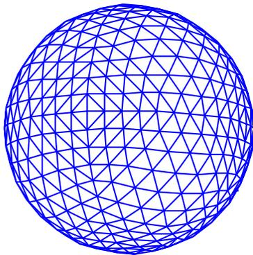
Fig.4 Example of a polyedral patch surface obtained from an 11-frequency tessellated octahedral triangle using the tripetal subdivision of the spherical triangle.
