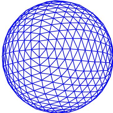
Fig.5 Patched polyedral surface obtained from an 11-frequency tessellated octahedral triangle using the concentric subdivision of the spherical triangle.
