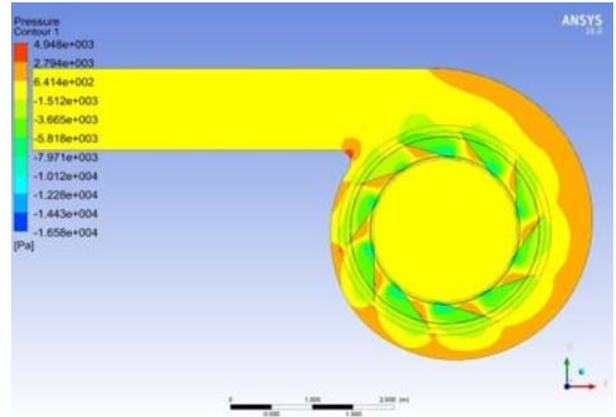
Fig 17: Pressure contour of 10 Blade forward Impeller
