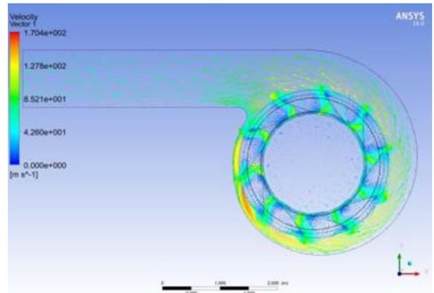
Fig 19: Velocity Vector of 10 Blade forward Impeller
