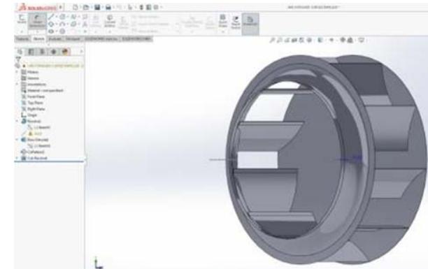
Fig 4: Forward Curved impeller with 10 blades
