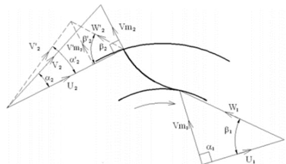
Fig 9: Theoretical and Actual Velocity Triangles as per fundamental Design
