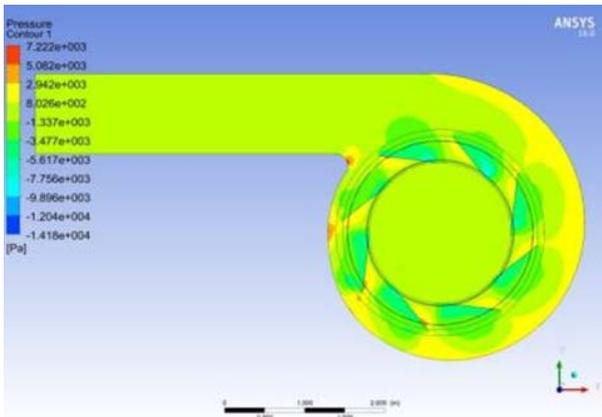
Fig 16: Pressure contour of 8 Blade forward Impeller
