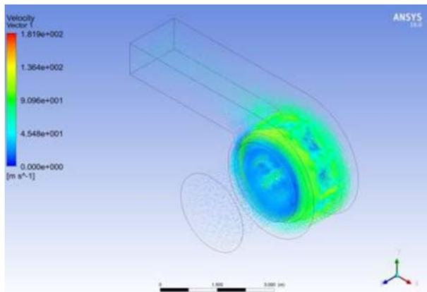
Fig 20: Velocity Vector Volume of 8 Blade forward Impeller
