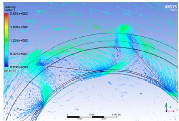
Fig 18: Velocity Vector of 8 Blade forward Impeller
