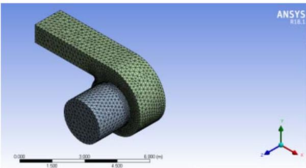
Fig 7: Mesh Model of Complete Fan with Ducts
