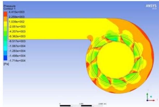
Fig 11: Pressure contour of 10 Blade forward Curved Impeller
