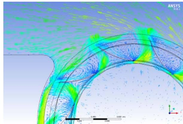
Fig 13: Velocity Vector of 10 Blade forward Curved Impeller
