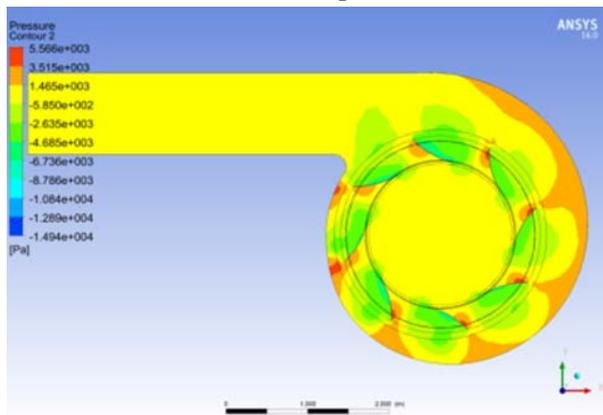
Fig 10: Pressure contour of 8 Blade forward Curved Impeller
