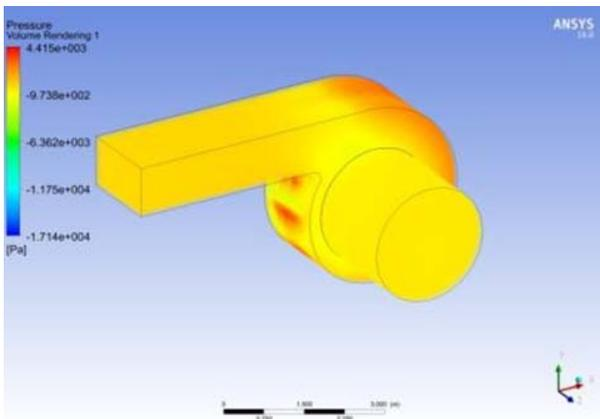
Fig 15: Pressure contour Volume of 10 Blade forward Curved
