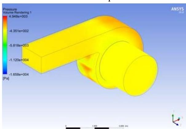
Fig 21: Pressure contour Volume of 10 Blade forward Impeller
