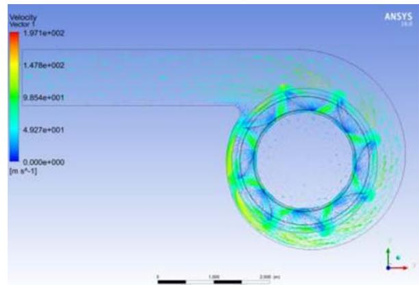
Fig 12: Velocity Vector of 8 Blade forward Curved Impeller
