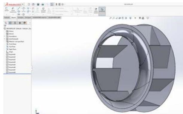
Fig 3: Forward Impeller with 8 blades ISO view
