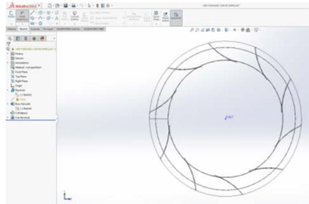
Fig 2: Forward Curved impeller with 10 blades front view
