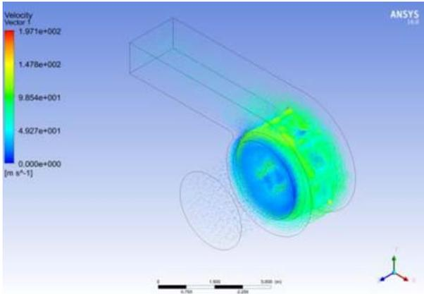
Fig 14: Velocity Vector Volume of 8 Blade forward Curved
