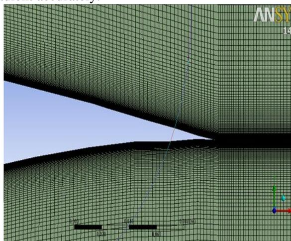
**Fig. 4. Mesh around trailing edge**
