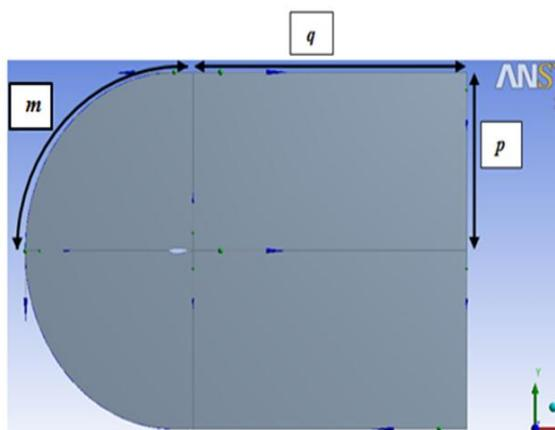
**Fig. 2. Geometry and dimensions of computational Domain**
