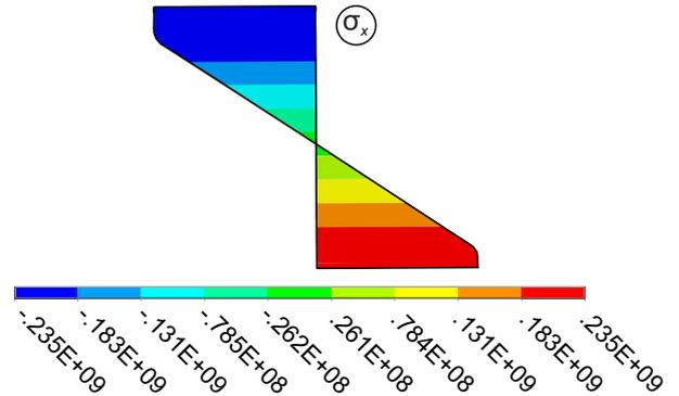
Fig. 10: Stress course in web  $\sigma_x$  for slenderness  $\bar{\lambda}_{LT} = 0.6$  at reaching the total resistance
