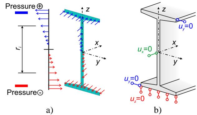
Fig. 3: a) Loading of edge cross-sections, b) boundary conditions
