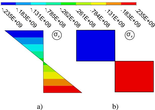
Fig. 9: Stress course in web  $\sigma_x$  at reaching : a) elastic resistance, b) plastic resistance
