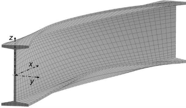
Fig. 4: Computational model in Ansys - axonometry
