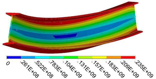
Fig. 11: Course of the von Mises stress  $\sigma_{vM}$  in the beam for  $\bar{\lambda}_{LT} = 0.6$  at reaching the total resistance
