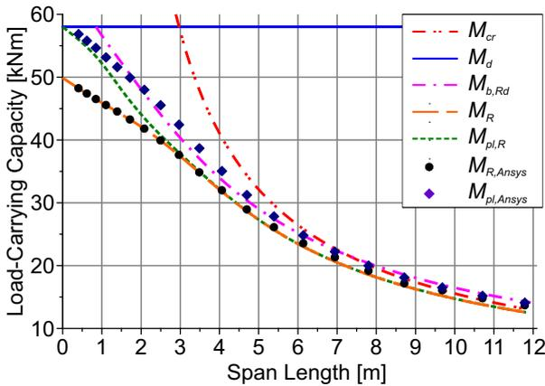
Fig. 8: Diagram resistance vs. span length
