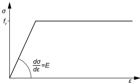
Fig. 6: Bilinear stress-strain diagram
