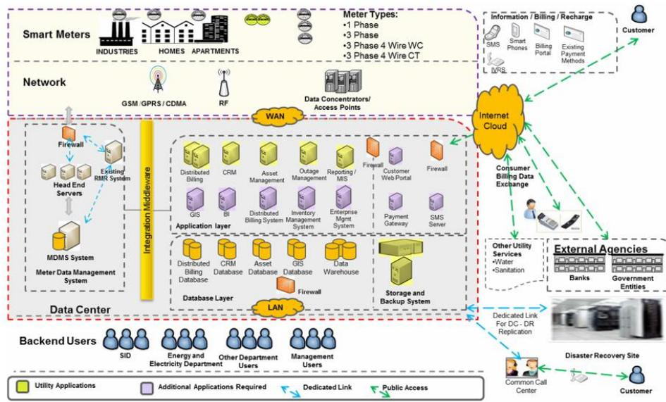
**Figure 5.** Smart Utility Meter Architecture with IoT [21]
