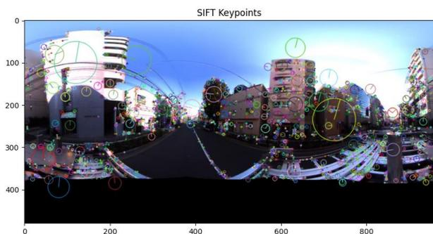
Fig. 2. Features extracted from omnidirectional image
