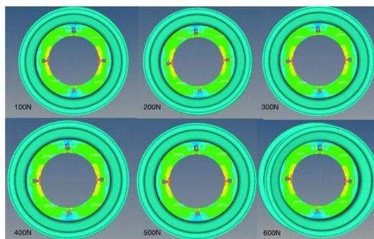
Figure Error! No text of specified style in document.: Finite Element Analysis results
