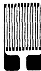
Figure 1: Wire resistance strain gauge (Roylance 2001)
