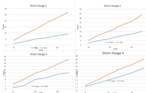
Figure 4: Comparison between FEA and test
