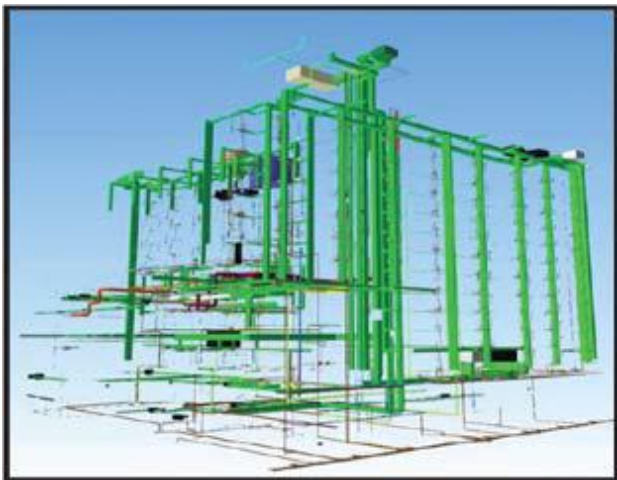
Fig.9: Plumbing model using BIM.
