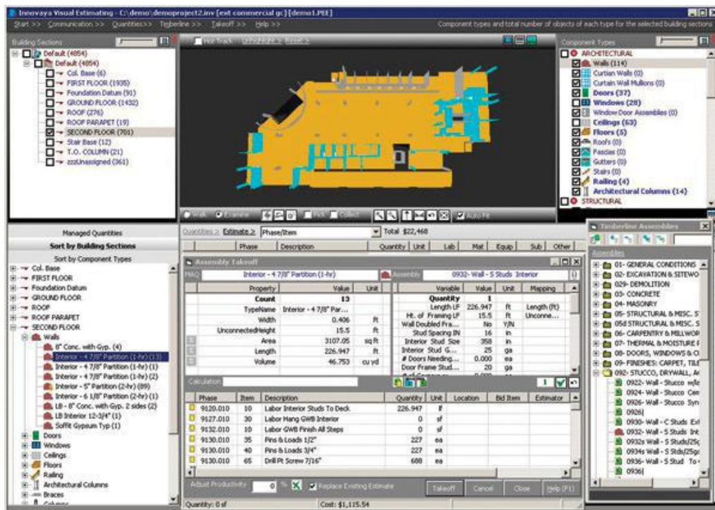
Fig.11: Addition of cost as a fifth dimension to the 3D model.
