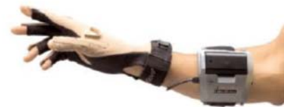
Fig. 2 Cyberglove II flex sensors based MCS (Cyberglove Systems image)
