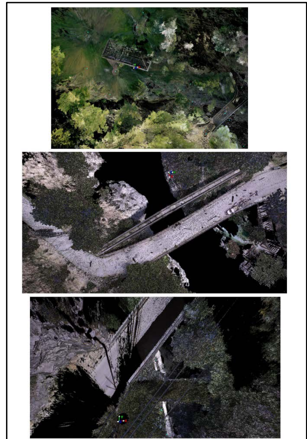
Fig. 11: Registration of scans for the three stone bridges.
