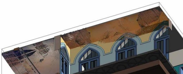
Figure 12: Deviations of the ceiling from the current state (measured point clouds) and the created digital model.
