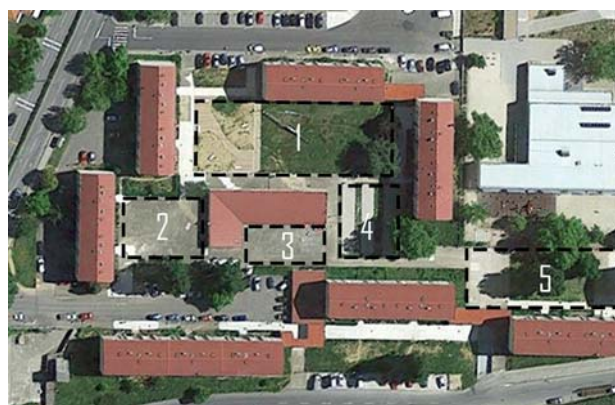
Fig. 6 – Final Design Programme specific objectives: (1) requalification of the clotheslines area, creating a green open meadows for multifunctional recreation, along with the clotheslines; (2) improving the green presence in the paved area and improve microclimate comfort; (3) requalification of the esplanade, adjusting the design to people’s stay and business
