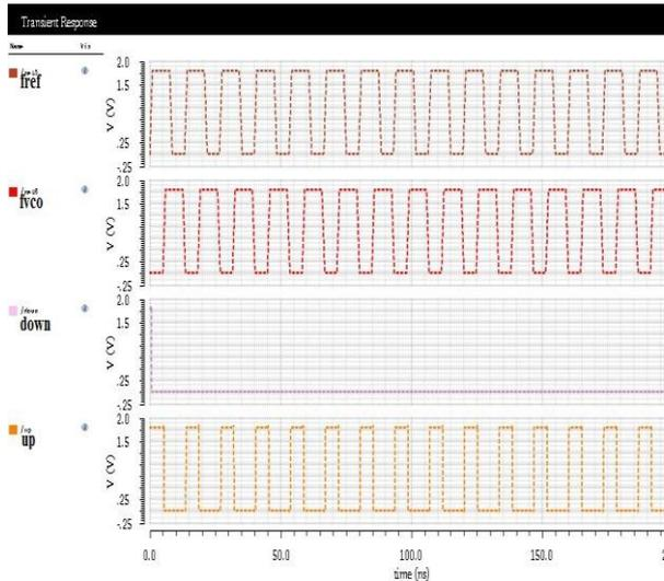
**Fig 7 Output of PFD when reference input signal is leading.**
