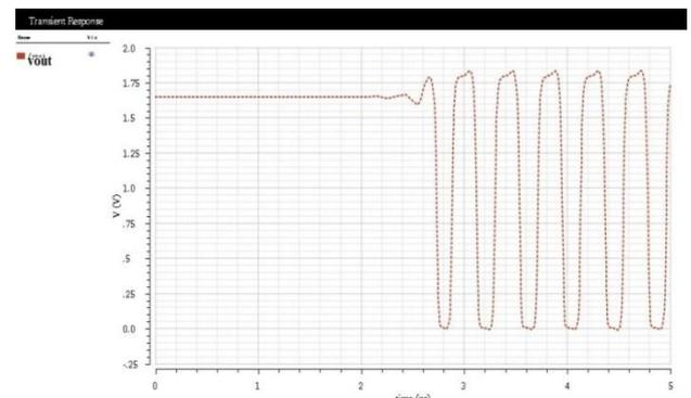
**Figure 18. RHBD VCO generating 2.4GHz frequency output.**
