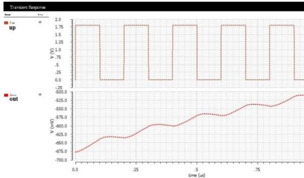
**Fig 11. Charge Pump output in presence of UP signal.**
