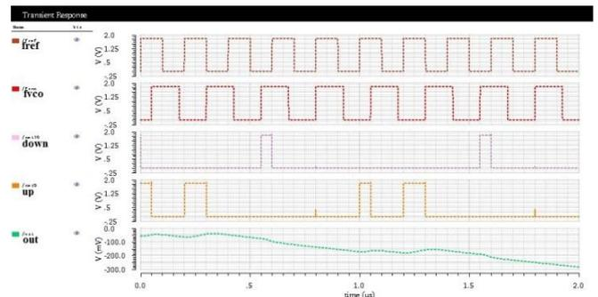
**Fig 16. Simulation Result of PFD with Charge Pump.**
