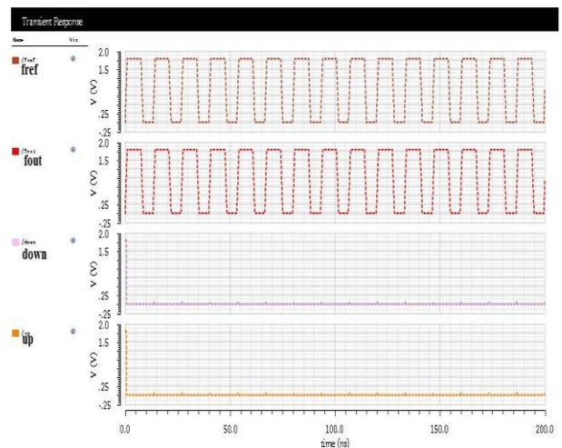
Fig 6 Output of PFD when inputs are in phase. When both the reference input and the feedback signal from PFD are in phase, both the outputs of PFD are zero.
