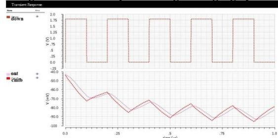
**Fig 15. CMFB output during Discharging cycle.**
