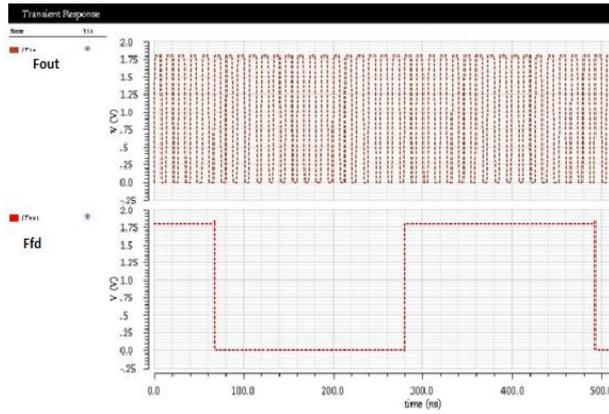
**Fig 21. Simulation Result of the Frequency Divider**
