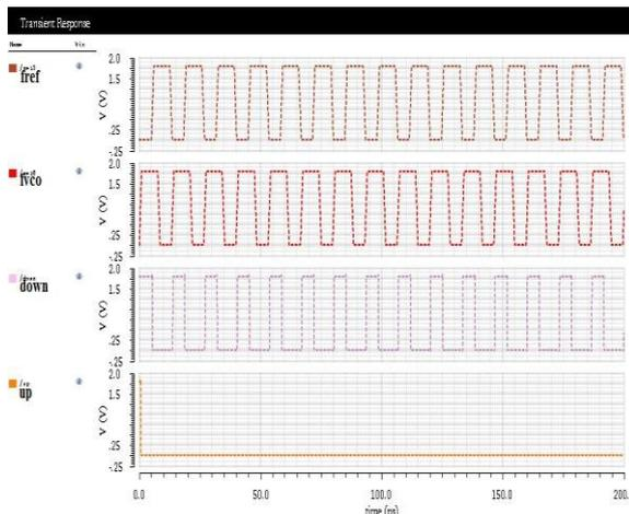
**Fig 8 Output of PFD when reference input is lagging.**
