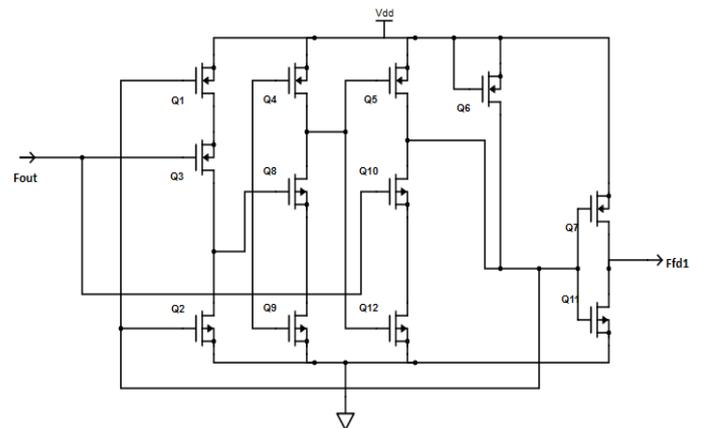
**Fig 20. RHBD Frequency Divider Circuit**
