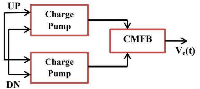
**Fig 9. Differential Charge Pump Circuit with CMFB**
