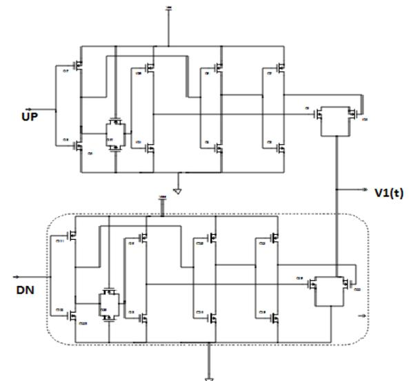
**Fig 10. Single Ended Charge Pump Circuit**
