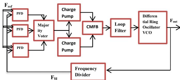
**Fig 2. Functional Block Diagram of Integer N RHBD Charge Pump PLL based Frequency Synthesizer.**
