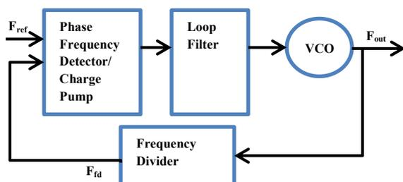
**Fig 1. Block Diagram of Integer N Charge Pump PLL based Frequency Synthesizer.**
