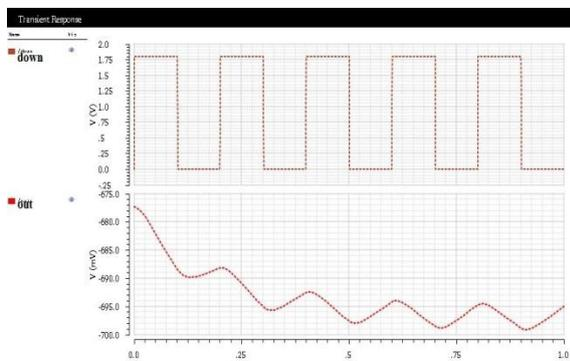
**Fig 12. Charge Pump output in presence of DN signal.**
