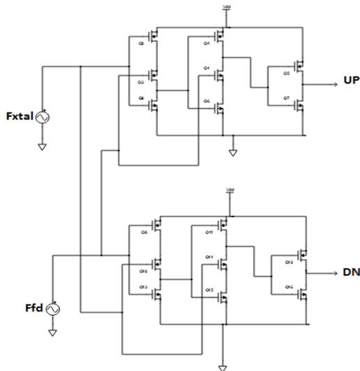
Fig 4. Schematic Diagram of the PFD
