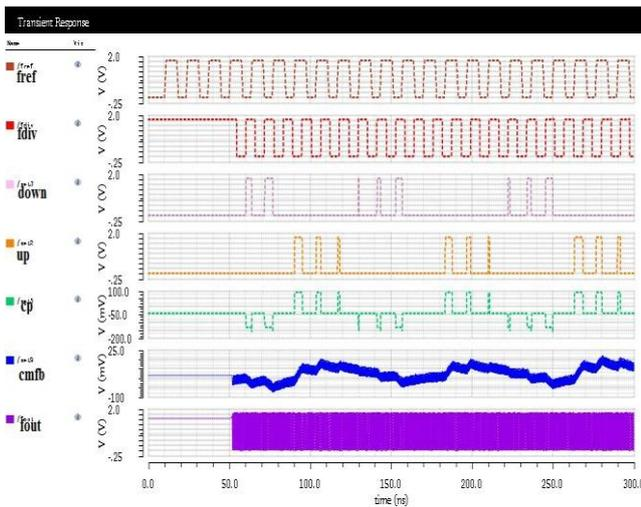
**Fig 22. Simulation result of the complete RHBD Charge Pump PLL circuit.**
