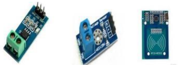
Figure 2. Front Panel Of Current Sensor, Voltage Sensor and RF ID Module
