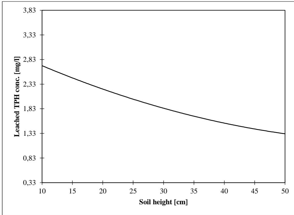
Figure 2: Leached TPH concentrations through varying soil depths.
