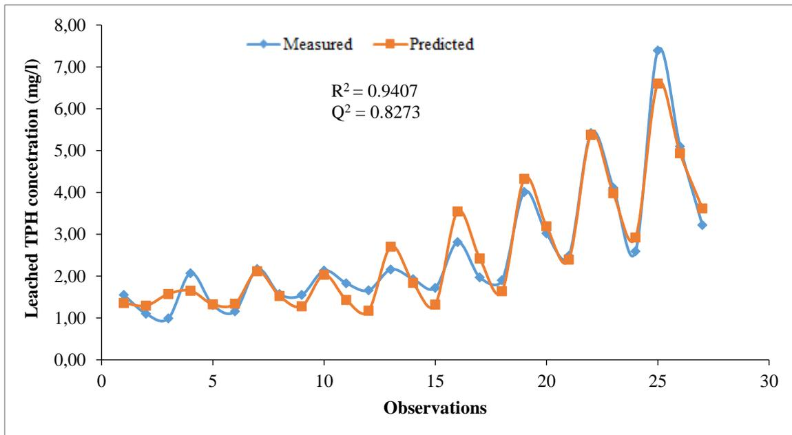
Figure 6: Comparison of measured and predicted leached TPH concentrations with different observation points.
