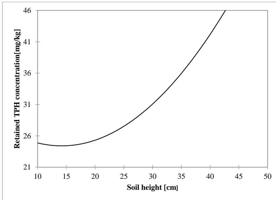
Figure 8: Retained TPH concentrations in varying soil depths.
