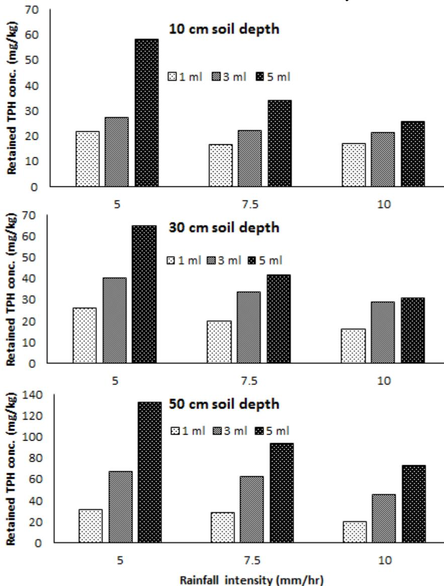
Figure 7: Retained TPH concentrations for various soil depths and rainfall intensities
