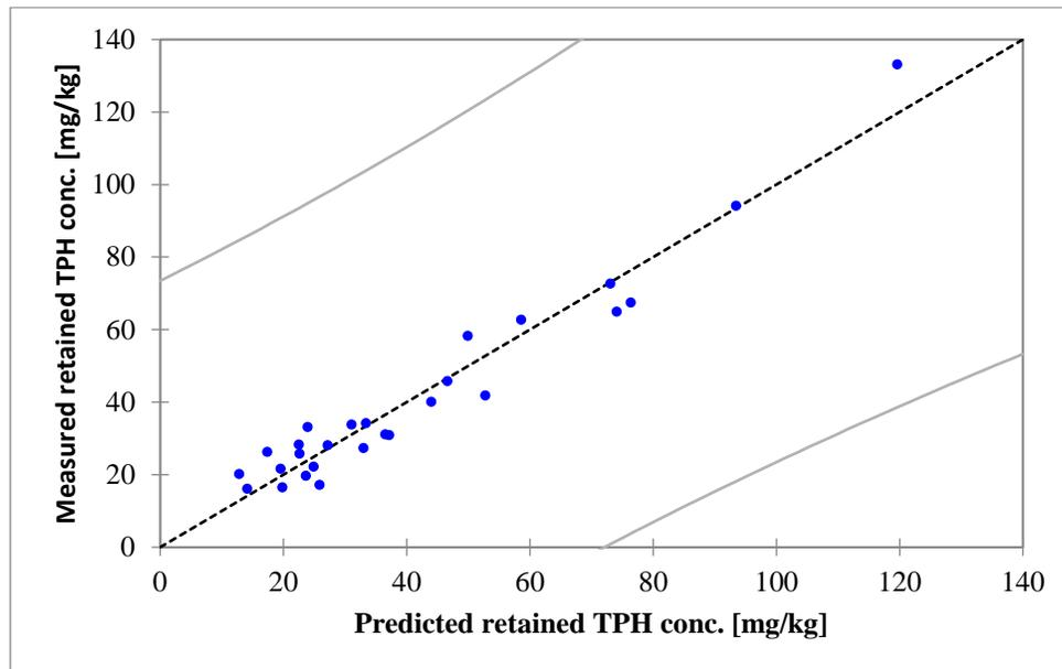
Figure 11: Relationship between measured and predicted retained TPH concentrations
