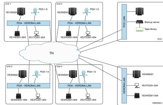
Figure 1: Connection of local VERONA networks to the technological network of the plant.
