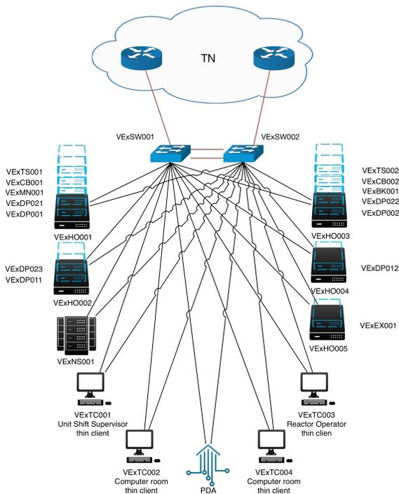
Figure 2: Local network of VERONA of a reactor unit.
