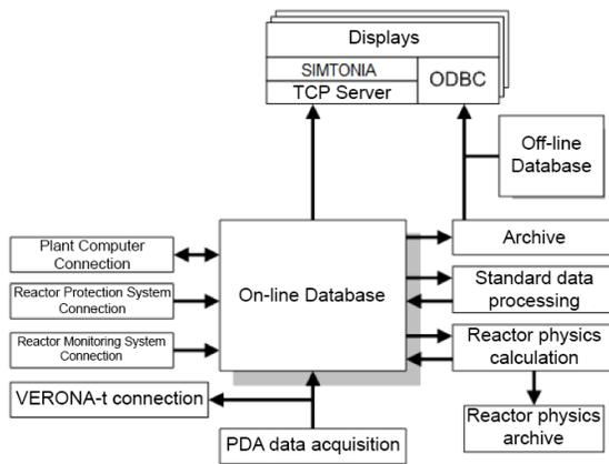
Figure 3: Connections of systems components in virtual VDP servers.
