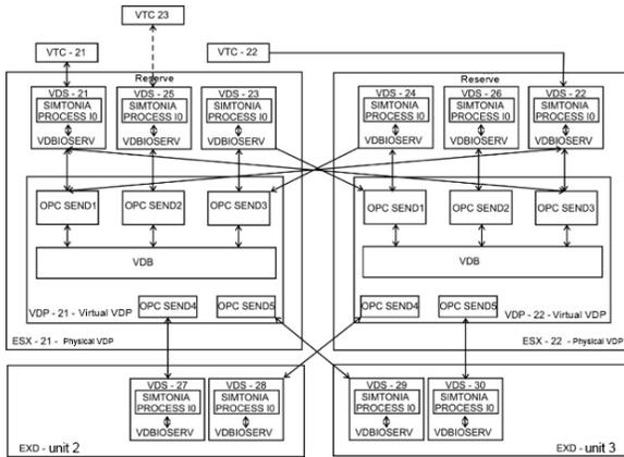
Figure 4: Connections of virtual display servers.
