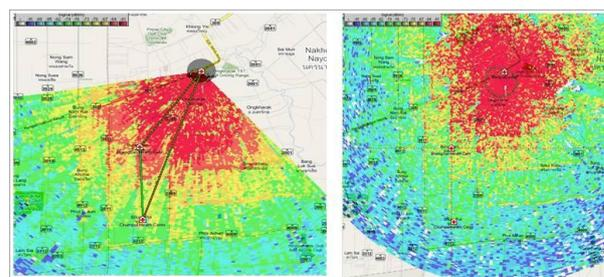
Figure 16. Radiation pattern of 3-sectors antenna system, the distance between the MSMC to two health sub-district
