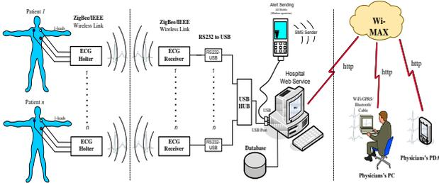
Figure 6. The structure of the signal processing system in the ECG monitoring
