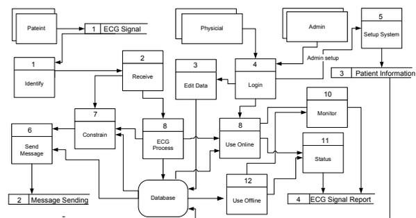
Figure 8. The Data Flow Diagram of ECG signal processing application
