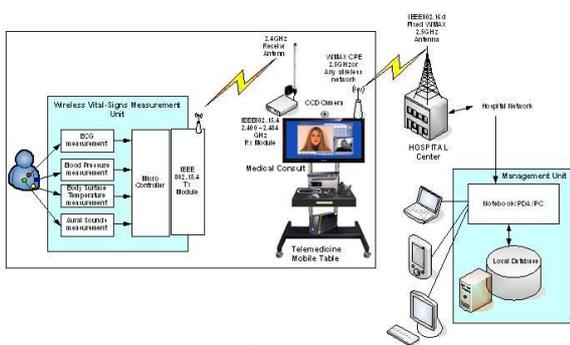
Figure 4. Structure of telemedicine via WBBN
