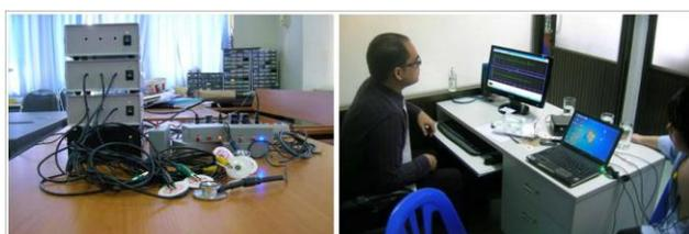
Figure 14. ECG&HS equipment prototype with monitoring via Wi-MAX network.
