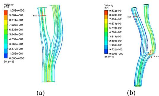
**Fig. 6.** Simulated velocities and localisation of measurement points for patient 1 (a) and patient (2).
