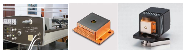
Fig 3. (Left a) the home-built-frequency-stabilized \text{CO}_2 laser with the larger size; (Left b) the small size Quantum cascade laser; (Right) Cooling Unit for HHL packaged QCL size (WxHxD) 68x82x117 mm.
