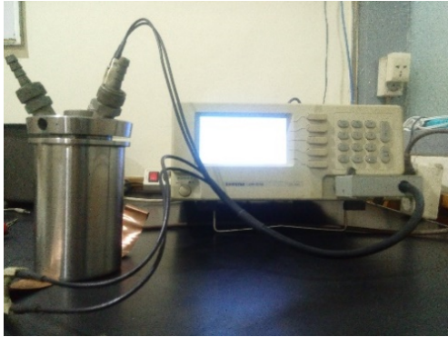
Figure 3. Liquid Test Cell and LCR Meter
