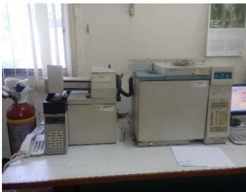
Figure 4. Gas Chromatograph HP 6890 integrated with Sampler HP 7649
