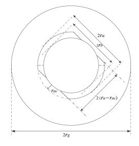
Fig. 1 Overhead view of the proposed antenna. The dimension of reactance element is included.
