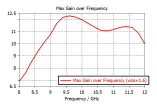
Fig. 10 Frequency characteristics of directive gain.
