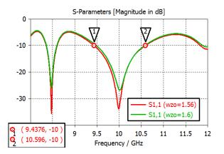
Fig. 9 Frequency characteristics of return loss.
