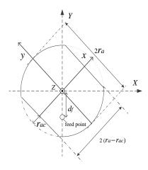
Fig. 3 Dimension of feeding element.
