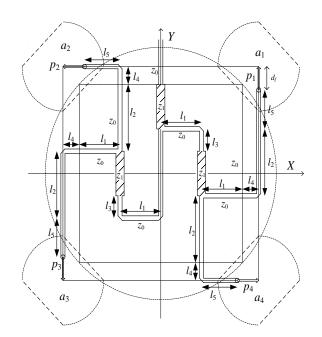
Fig. 8 Routing wire pattern for the proposed array antenna with 4 unit antenns.
