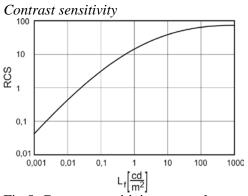
Fig.5. Contrast sensitivity versus the Background luminance
