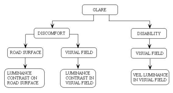
Fig. 6. The evaluation of glare in traffic road
