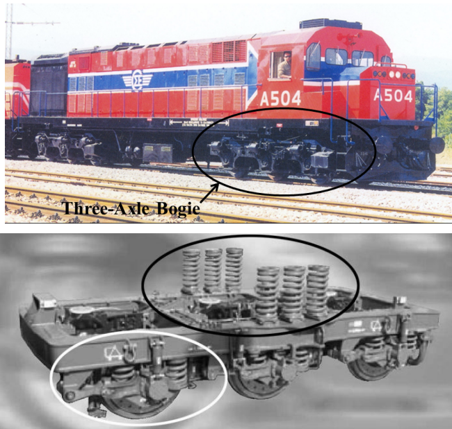
Figure 2. (Upper illustration) MLW 500-series diesel locomotive of the Greek railways, with three-axle bogies; the three-axle bogie is marked with the black ellipse. In Greece, Q_{\max} 22,5 t/axle and NSM_{\max} 5,08 t/axle. (Lower illustration) A three-axle bogie in detail: in the white ellipse the primary suspension and in the black ellipse the secondary suspension are depicted.
