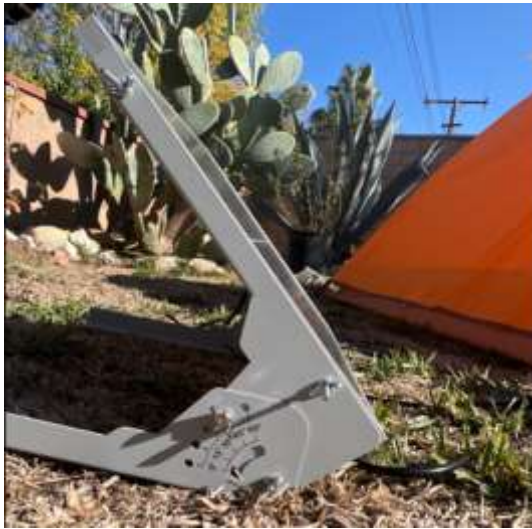
Fig. 6 Side-view of solar panel stand with title angle selection (45° selected)
