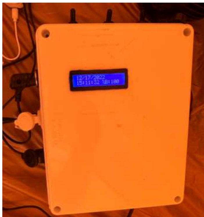
Fig. 8 Junction box with LCD Display, DC Cigarette outlet, USB outlets and manual switches
