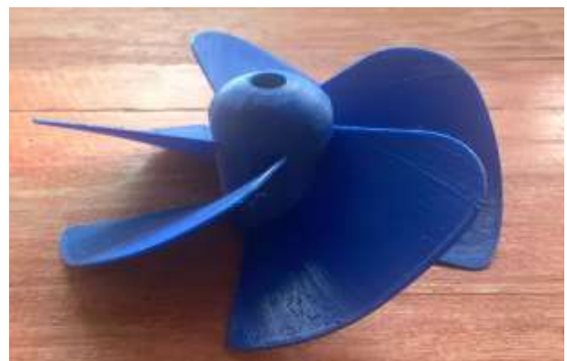
Kaplan turbine runner in figure 3.
