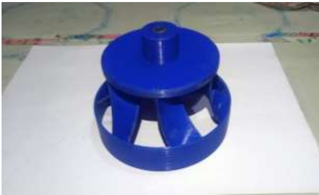
Francis turbine runner in Figure 4.
