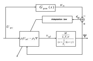
Figure 1: Diagram block in closed loop of MRAC regulator of flux.
