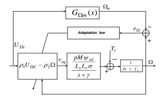
Figure 2: Diagram block in loop closed of MRAC regulator of rotating speed .
