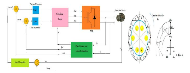
Fig 1. Structure of classical DTC by neuronal
