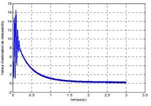
Fig.11. DTC-ANN control with KUBOTA observer to estimate the speed
