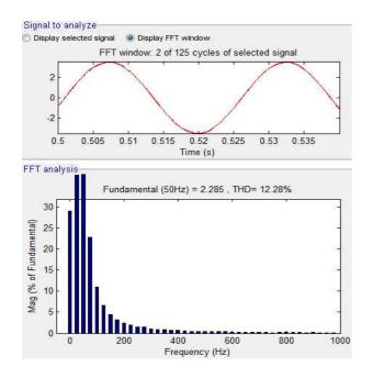
Fig17. THD value of stator current of DTC-RNA.
