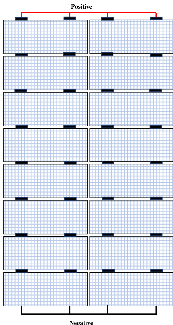
Figure 8: GaAs solar array layout.
